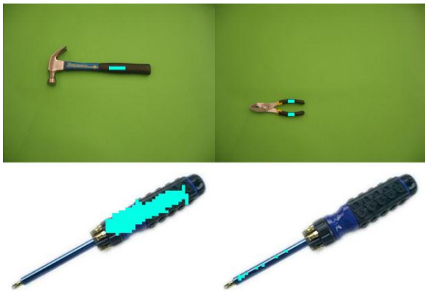
Fig. 3. Two Goals of object purpose based grasping: the upper 2 images demonstrate the goal of effectively infer grasping points of objects in any category; the lower 2 images demonstrate the goal of being able to infer different grasping points based on different purposes of the same object: the grasping point on the left is of a screwdriver used as a screwdriver, while the grasping point on the right is of a screwdriver used as a hammer.
